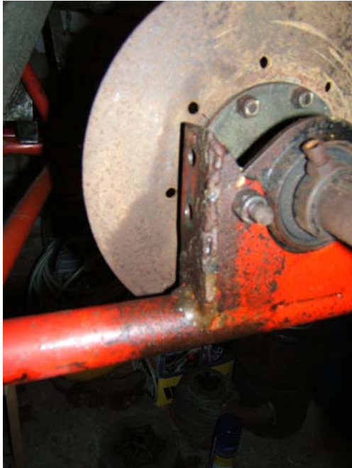
Two bolt bearing hangers with 45 degree flange stiffeners on the supports, horrible mechanical disc with messy home welded bracket for it indicating that originally it probably had a drum brake.
